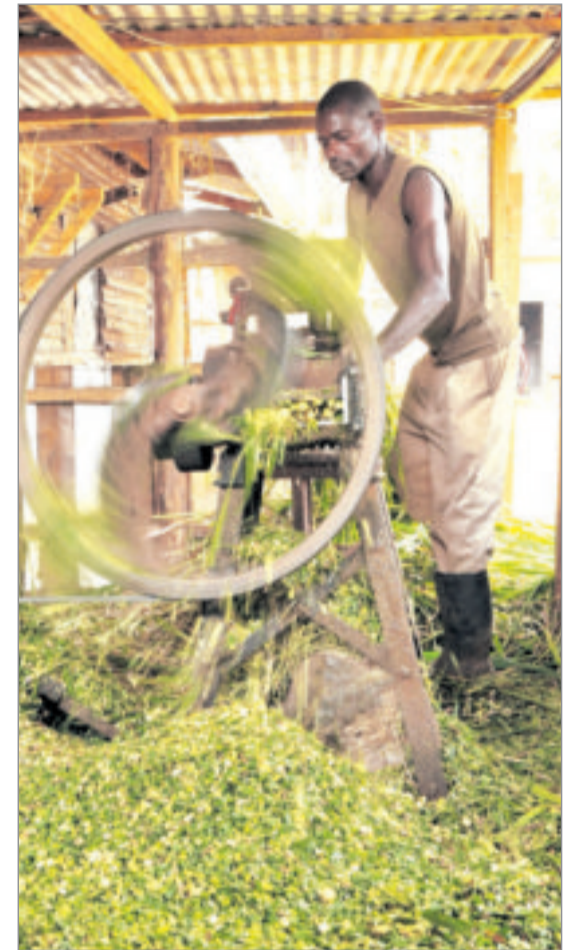
Macharia in Kieni East powers the chaff-cutter with electricity produced from biogas to cut Napier grass for fodder. PHOTO: UNDP-GEF/Small Grants Programme
