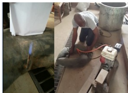
From left, Blue Gas Flame; next, Two Stroke ICE being Powered by the Gas Generated from the Pyrolysis Process (Photo credit: Fritzi Ziebel and Eugene Sefa-Appiah)
