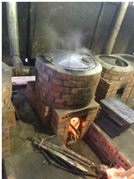
Photo above: Efficient Biomass Cookstoves with Chimney and below, Improved Fish Smoker Built by Commeh and Associates (Photo credit: Michael Commeh)
