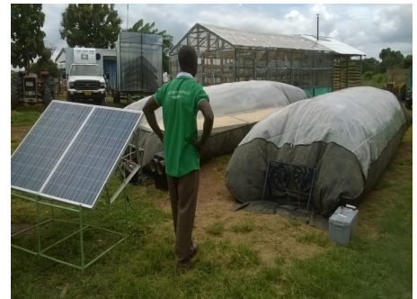
Solar-Gas Hybrid Mobile Dryer (above) and Solar Biomass Hybrid Dryer (below) developed by PENS Food Bank
