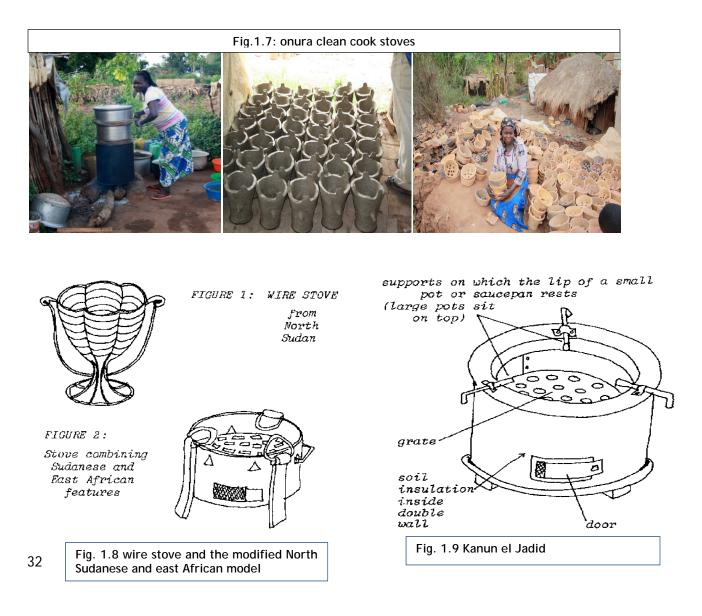
The improvements are in the insulated walls filled with earth and the placement of the saucepan into the firebox. The soil insulation reduces heat loss by directing it upwards onto the base and sides of the lowered saucepan.
