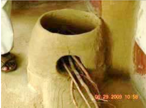
Figure 3.1: CSIR-IIR Improved Firewood Stove
