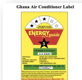
Figure 4: Air conditioning label (The number of stars corresponds to the level of efficiency)
